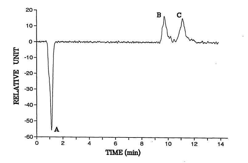
noise level became larger with increasing mobile phase viscosity. This problem was solved by touching the column end to the tip of a drill bit to direct the liquid flow. The baseline stability in our work was found to be limited by the residual fluctuations at this interface.
