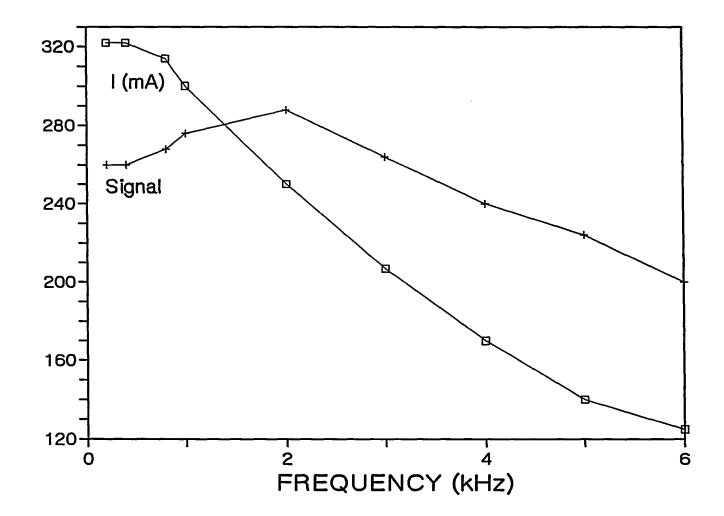
Fig. 2 and Fig. 3 showed similar dependence of signal on current. These results indicate that it is the ohmic heat,  $I^2R$ , generated in the solenoid at high currents that caused a decrease in signal.
