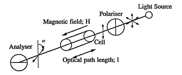
Figure 1. The Faraday effect. The magneto-optical rotation  $\alpha$  depends on the property of the substance inside the cell, magnetic field strength and cell path length
