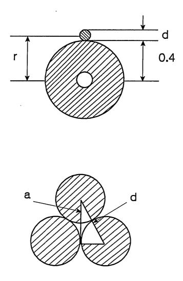
Figure 1. Cross-section of the solenoid. r, inner radius; a, layer thickness; d, wire diameter.
